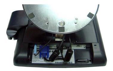
• Connect one end of the **speaker cable** to the speaker port in the computer and the other end to the port in the monitor. After connecting the speaker cable, secure it under the cable management clip.
